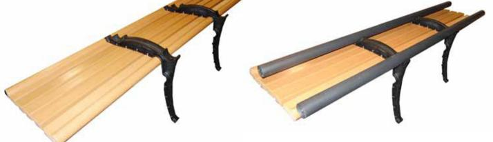
Arrange seat on a clean flat elevated surface. Place the *end slats*, rounded side facing outward and upward on each end. Align the *center supports* with the pre-drilled holes on the underside of the slats. Install the *center supports* using a philips screwdriver and the 1" philips screws provided. All of the screws may be tightened at this step. Take care to keep the ends of the slats aligned. Place the *support rods* in the channels on the *center supports*.
