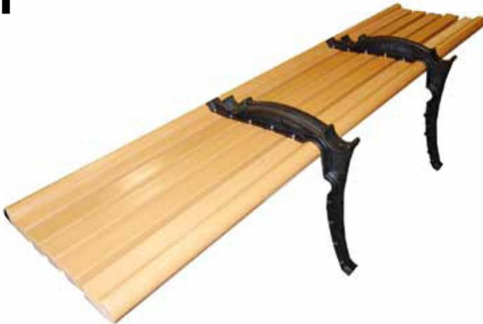
Arrange seat on a clean flat elevated surface. Place the *end slats*, rounded side facing outward and upward on each end. Align the *center supports* with the pre-drilled holes on the underside of the slats. Install the *center supports* using a philips screwdriver and the 1" philips screws provided. All of the screws may be tightened at this step. Take care to keep the ends of the slats aligned.
