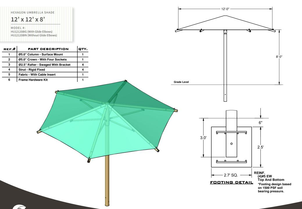
These drawings are for reference only and should not be used as construction details. Materials, fasteners, and foundations are subject to change if professionally sealed engineering drawings are required. Designed for 93 MPH Basic Wind Speed.
